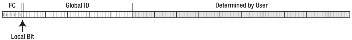
Figure 4-6. The unique site local IPv6 unicast address format
